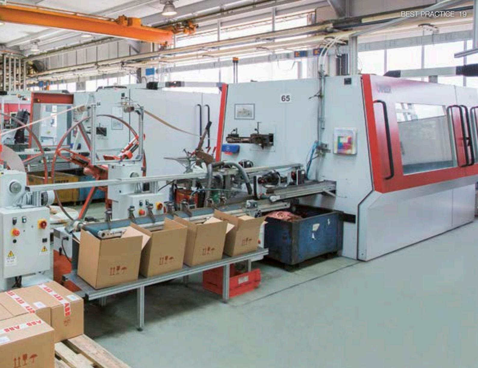
The moving contacts for the circuit breakers are manufactured on two GRM 80P stamping and bending machines. At 200 parts per minute on each machine, throughput is around three times as high as with alternative techniques.
