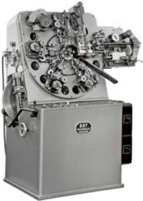
The starting point for decades of success: The world's first radial wire and strip bending machine developed in 1955/56 by Otto Bihler.
