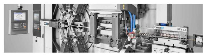
Components with welded-on contacts for industrial switching technology can be produced efficiently using stamping and forming technology - at very high speed and consistently high quality. These contact components are used in many industries: from information technology and control engineering to low-voltage, medium-voltage and high-voltage technology.
