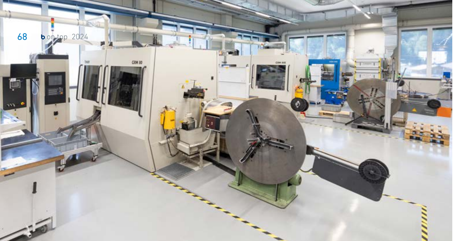
At Wörgartner, a total of 27 Bihler systems manufacture complex stamped-and-formed parts in a material-efficient and finished manner.
