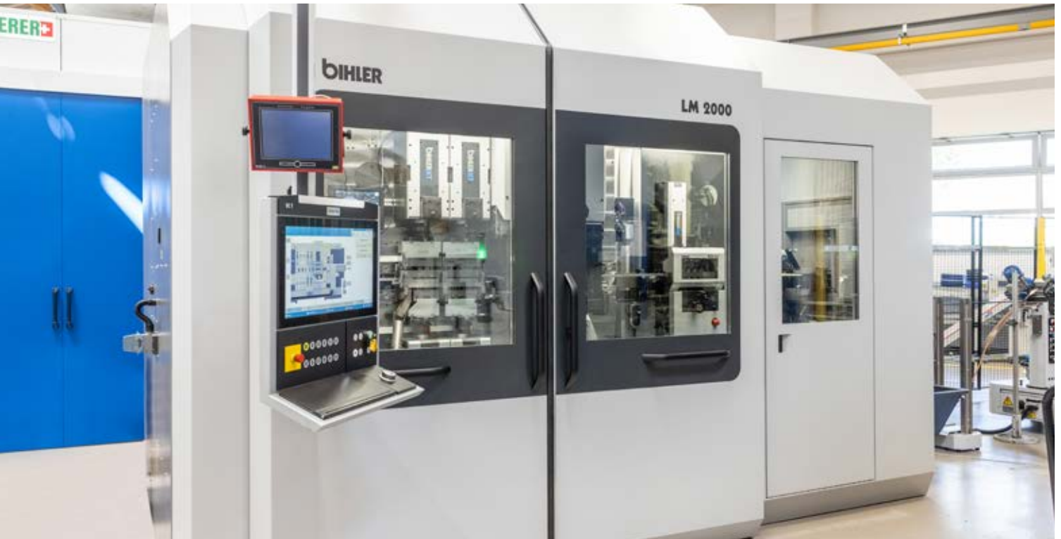
New high-performance machine: The DRÄXLMAIER Group uses the Bihler LM 2000-KT to manufacture box terminals for boards at a rate of approximately 400 strokes per minute.
